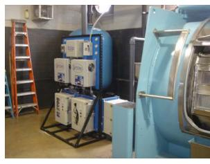
*OZONE* carries an electrical/chemical charge in the washing solution, which actually starts to dissolve soil on contact. This process activates the chemicals in cold water instead of using hot water at 140-160 degrees.
